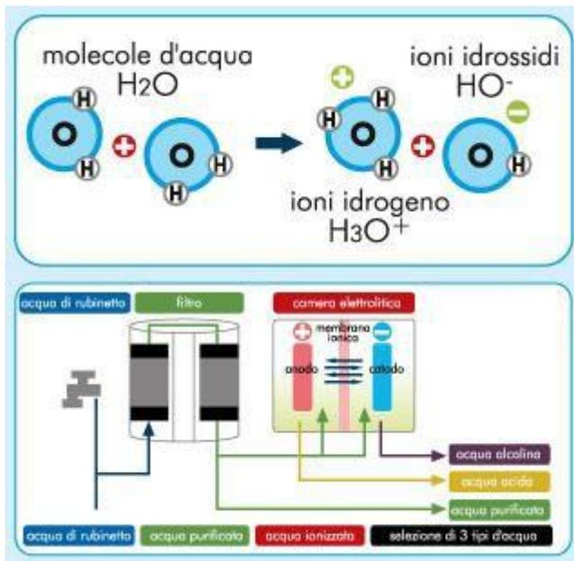
At the same time, negatively charged acidic minerals (chlorine, nitrate, sulfur, etc.) are pushed through the selective membrane into the other half of the ionization unit. In alkaline water OH- ions are formed and it is free of positively charged hydrogen (H+). A part of this positively charged hydrogen is released in the form of hydrogen gas bubbles in the glass, producing a slightly turbid-lacquid color that disappears in a short time.
