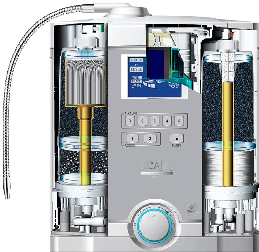
The ECAIA Filter No. 1 is designed to remove especially harmful heavy metals. At the inlet the water immediately passes through the sediment filter, thus starting the purification process. Here the coarsest material and rust staining is removed.
